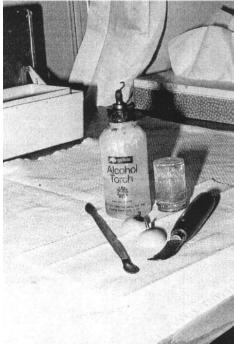
Figure 2. Tools required for designing a wax fitting shell include a wax carving knife, alcohol torch, and wax spatula.
