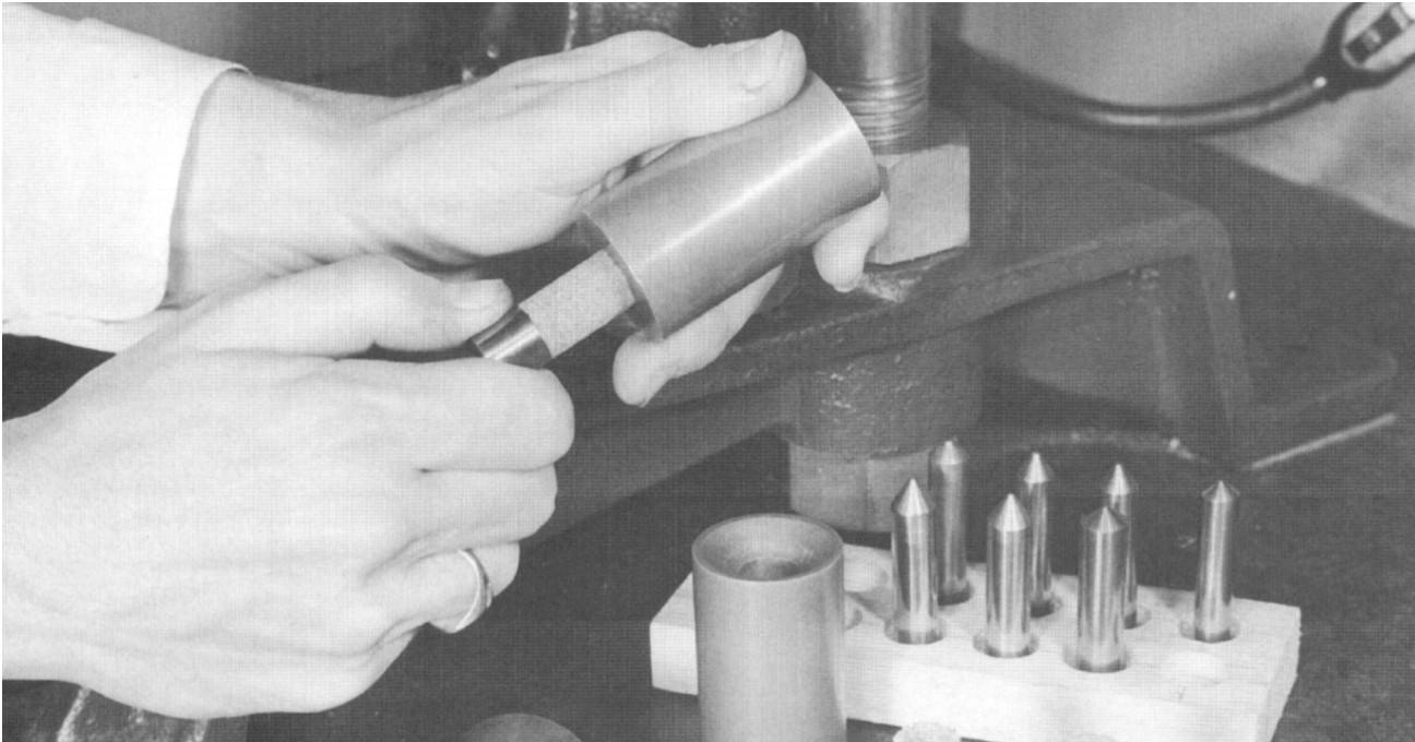
FIGURE 2 Using a steel die, the main body of the iris is cast using acrylic pellets. The acrylic is cured using a Carver hydraulic press.
