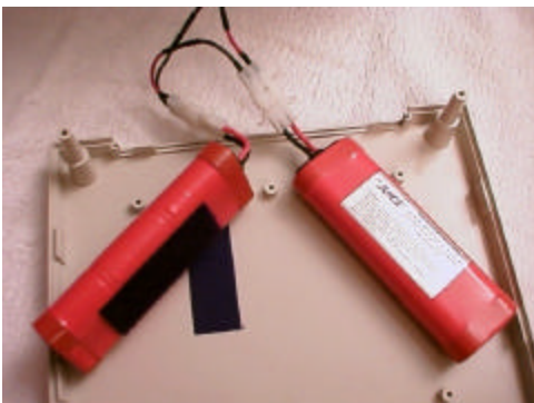
Figure 3 Battery Pack with Velcro provide security.
