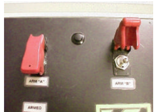
Figure 6 Arming Switches & Test Button
