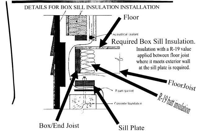
The above side view cross section shows the area of the box sill that must meet a minimum R-19 value for a FmHA Rural Development Loan on an existing dwelling.
